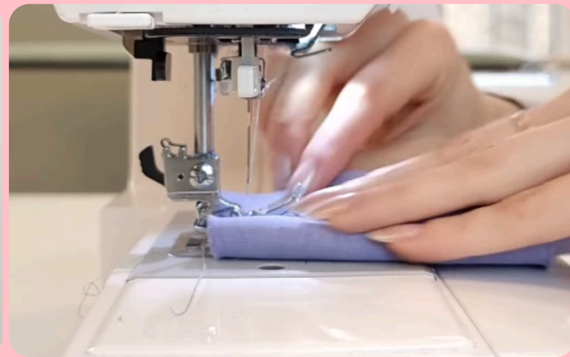
Place The Basted Layers Under The Presser Foot
